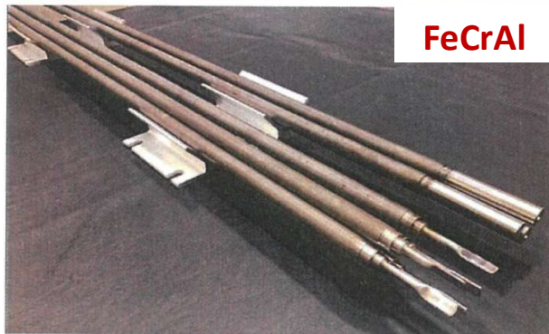
Fig. FeCrAl alkali metal heat pipe for high operating temperature
